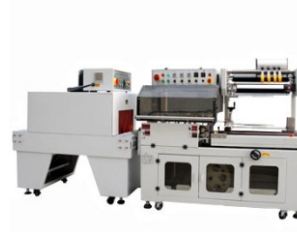
Fully Auto L- Sealer With Shrink Tunnel
